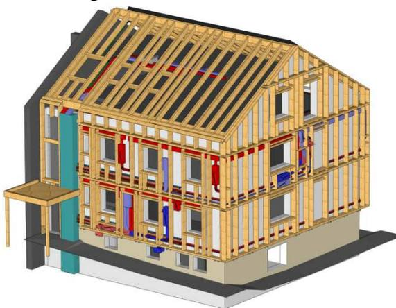
Figure 1.a) air distribution ducts and MVHR units integrated in the insulated timber frame envelope.
