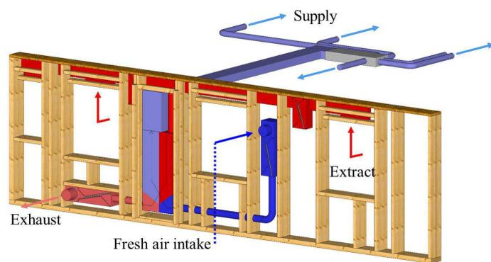
Figure 3.b) Scheme of the components and ducts of KIT 1 (Source: Gumpp & Maier GmbH)
