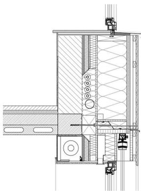
Figure 3.a) Detail showing the position of pipes, ducts and inlets in the layer between the old and the new walls (Source: Gumpp & Maier GmbH)
