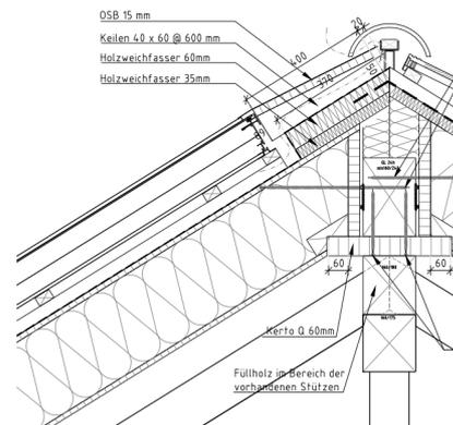
Figure 5.b) In roof integration of the collector (Gumpp & Maier GmbH)
