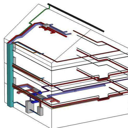
Figure 1.b) vertical distribution shaft with the water and electrical lines around the existing building together with a solar collector.
