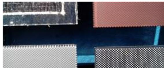
**Figure 3:** Close-up photo of the various CIGS panels of the prototype demonstrator. At the top left the black textured glass panel is depicted, at the top right the printed red panel, at the bottom left the printed grey panel and at the bottom right the grey foil panel.
