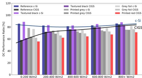
**Figure 10:** Performance Ratio results of all PV panels in 200 W/m<sup>2</sup> irradiance bins.
