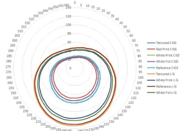
**Figure 12:** Simulation results for PV façades located in Amsterdam, of various PV technologies and orientations with various colors and textures. The annual yield is in kWh/m<sup>2</sup>
